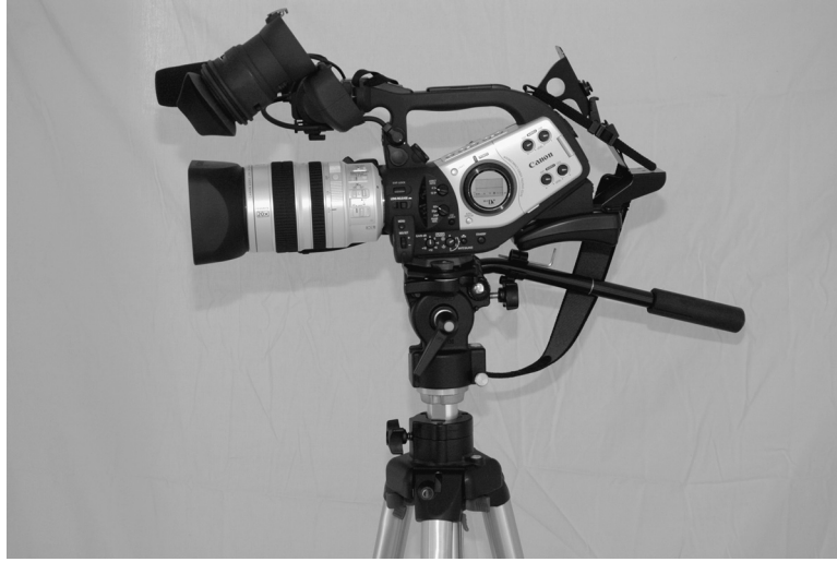
Photo 11.1 This portable three-chip digital camcorder is less than 9 inches wide, less than 9 inches in height, and under 20 inches long (with the lens). Its total weight is under 8 pounds.
